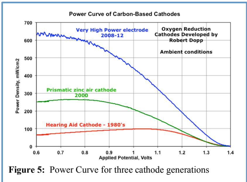
**Figure 5:** Power Curve for three cathode generations
