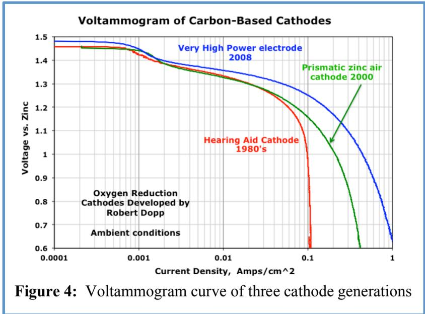
**Figure 4:** Voltammogram curve of three cathode generations
