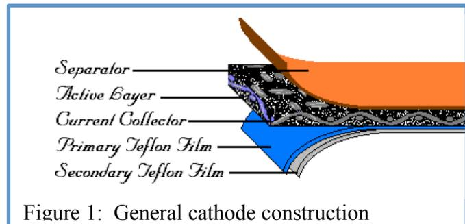
Figure 1: General cathode construction
